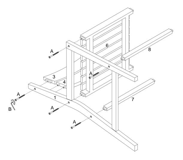
Using bolt (A) attach part (1) to parts (3,6,7,8) with hex key (B), attach part (4) to part (1) as per diagram.
