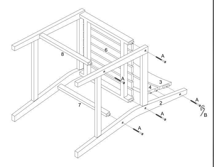
Using bolt (A) attach part (2) to parts (3,6,7,8) with hex key (B), attach part (4) to part (2) as per diagram.
