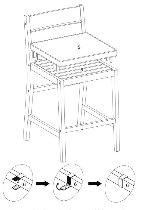
Place part (5) as per diagram, then tighten the Velcro to part (6) as per diagram.
